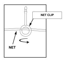
Twist net until it snaps into position. Net must be centered through clip.
